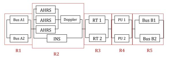
**3)** At the high-level we can consider the system as the series of 5 main components shown above: Bus A, INS/AHR, RT, PU, and Bus B. So we can write the high-level reliability formula as:
