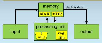
The LC-3 has one **input** device: **a keyboard**. And one **output** device: **a monitor/display**.
