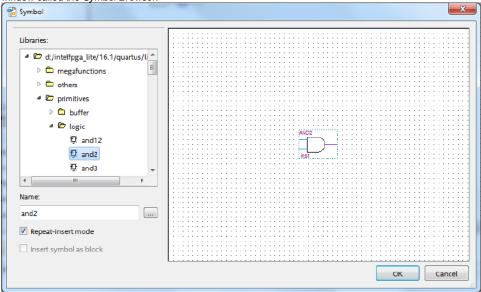
b. In the Libraries section of the Symbol Browser navigate to find the 2 input AND gate (under primitives/logic section) as shown above. Click on and2 and then click OK button. You will be returned to the schematic window and your mouse cursor will look like an AND gate. Place this gate as shown below. Click Esc keyboard key to exit from this mode.
