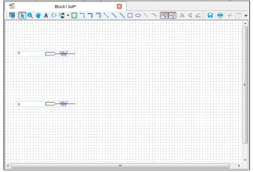
4. Add an output port. Click on the **Pin Tool** drop-down menu at the top and select **Output**. Place a single output port on the right side of the schematic window and edit its label.
