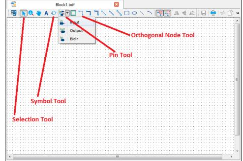
3. Your mouse cursor will change to *input port* symbol. Add two input ports, by clicking on two different places on the left side in the schematic window. Then press **Esc** button on your keyboard to exist from the **Pin Tool** mode. Edit port labels; your final result should look as follows:
