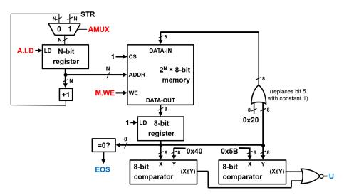
Inputs for use by external logic, including the STR input, are shown in black. Datapath control signals appear in red. Datapath outputs are shown in black.
