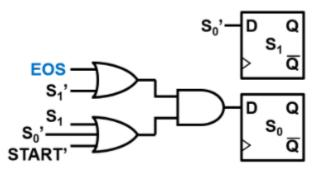
a) The system starts in a WAIT state (S<sub>1</sub>S<sub>0</sub>=01), allowing external logic to write a string into the memory (logic not shown). The external logic provides the starting address of the string through the STR input and raises the START input to make the FSM change any upper-case letters in the string to lower case.
