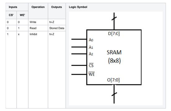
The following chip is a 8x8 bit RAM. Its logic symbol and function table are shown below:
