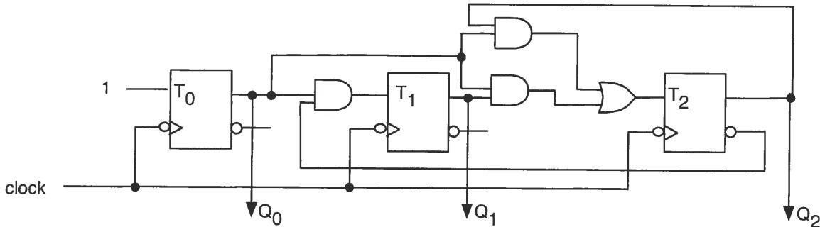
1. (5 points) Give Boolean expressions for the  $T_2$ ,  $T_1$ ,  $T_0$  flip-flop inputs, each as a function of the state variables  $Q_2$ ,  $Q_1$ ,  $Q_0$ .
