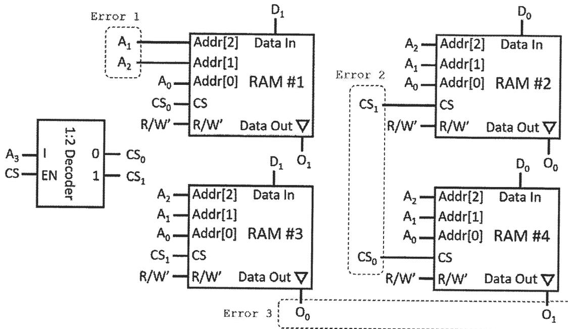
1. (12 points) Suppose a user attempts to write ( $CS=1$  and  $R/W'=0$ ) into the faulty 16x2 RAM with data  $D_1D_0 = 01$  at address  $A_3A_2A_1A_0 = 0101$ . Indicate in the table below which of the 8x1 RAMs are accessed by **circling YES or NO** for each RAM. If an 8x1 RAM is accessed, also write down the 1-bit Data-In and the 3-bit address  $Addr[2:0]$  for that 8x1 RAM.
