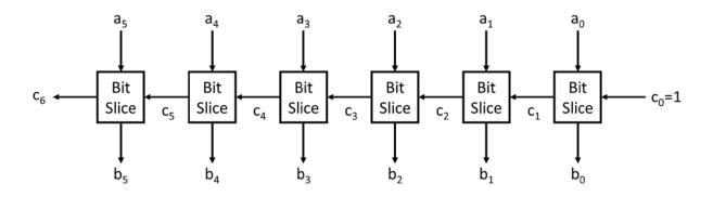
**1. (8 points)** Each bit slice is identical. Complete the truth table for a single bit slice and write the minimal SOP expressions.
