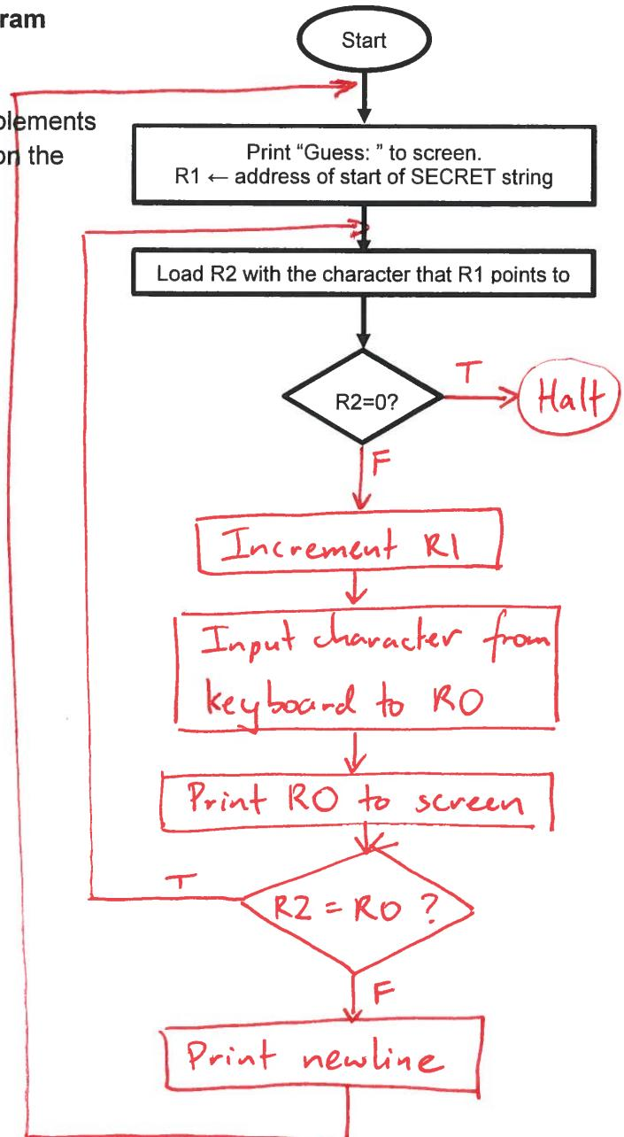
2. (10 points) Write down exactly what this program prints to screen when the user runs the program and enters **BITBYTE** using a keyboard. Note that GETC inputs a character from the keyboard but does not print anything to the screen.
